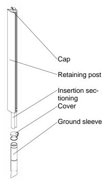
**Wall holder:** screw the wall plate approximately 985 mm high on the wall and mount the wall holder using the cylindrical SW4 screws.
