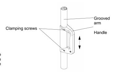
3.7 Set its height so that the awning is tensioned dead straight.
